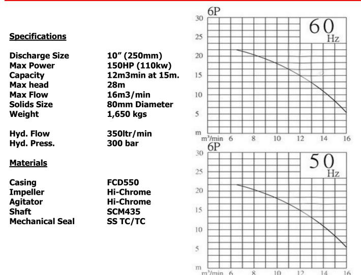
The main features of our heavy duty slurry pump is a heavy design of wear resistant casing and 28% HiCr impeller. Excellent combination of materials provides long term operation even in harsh abrasive slurries.
